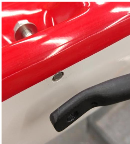
You can now press the backstay against the boat and line it up with the hole. The backstay will likely have some tension in it which you can relieve by tapping the middle of the stay towards the boat a couple of times. This will help the backstay line up properly with the bolt.
